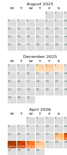
Flooding risk (99th percentile threshold) 1.34m above tide gauge zero
