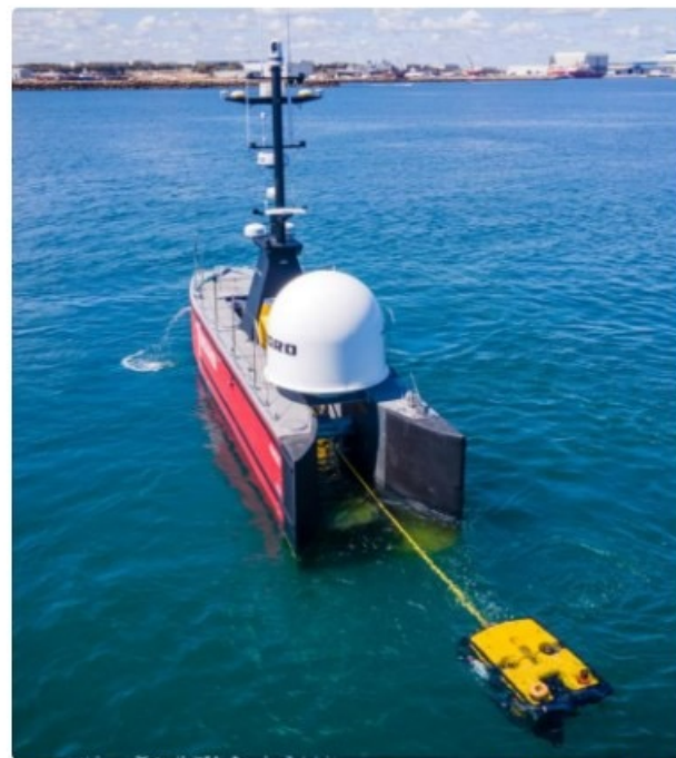
The USV with a remotely operated vessel (ROV) attached.
