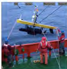
FIG. 1. Wave glider SV3-151 being deployed from the ARSV Laurence M. Gould near the Antarctic Peninsula.
